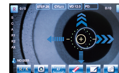
When move the device into the range of the patient's eye socket, it will track down a measuring focus of the eye automatically by the light sensors and 3D mechanism system inside(AF mode)
